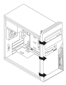
Figure 6. Removing the front bezel
